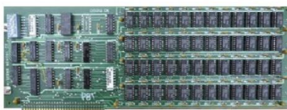
Random Access Memory Module (Less formally called a Board or Card)
