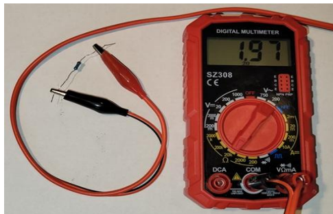
Image – Measuring a 2K \Omega resistor
