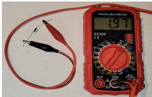
Image – Measuring a 2K \Omega resistor
